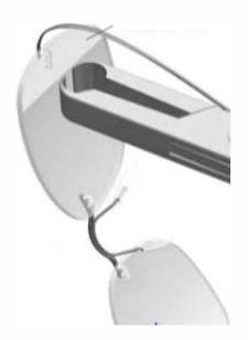
3) Gently pull sleeve and frame post from the lens You can use a back and forth gentle rocking to slowly pull it out. As long as you have CAREFULLY and COMPLETELY cut the exposed part of the compression fitting, it will workout. often tools will have two small metal rods to help push any remaining material out of drill holes:
